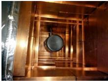
Figure 1: The cavity of the CUBED low-background counting station
